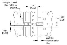
Dimensions are in Inches [Millimeters] X3DC35P1S Mounting Footprint
