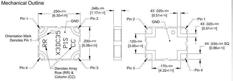
Dimensions are in Inches [Millimeters] X3DC35P1S Mechanical Outline
