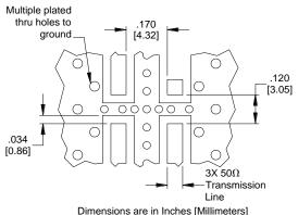
Dimensions are in Inches [Millimeters] X3DC25P1S Mounting Footprint
