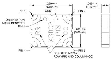
Dimensions are in Inches [Millimeters] X3DC21P1S Mechanical Outline
