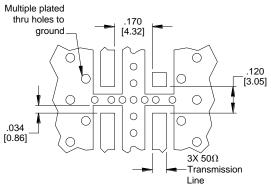
Dimensions are in Inches [Millimeters] X3DC21P1S Mounting Footprint
