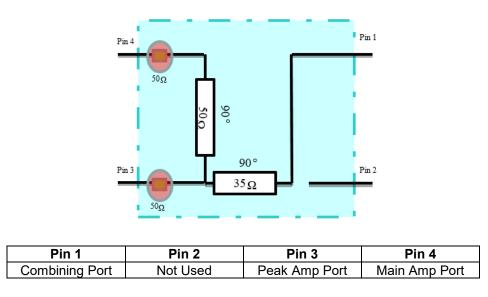
There are inevitably short lines associating with input ports in some high frequency band parts. The length of the short line is specified as electrical length at center frequency and noted as port extension in this datasheet. The designer should take this length into the consideration to optimize the offset line length.
