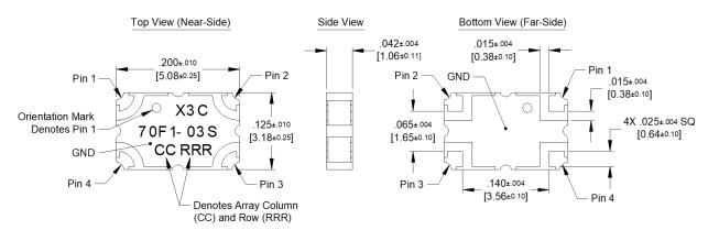
Dimensions are in Inches [Millimeters] X3C70F1-03S Mechanical Outline
