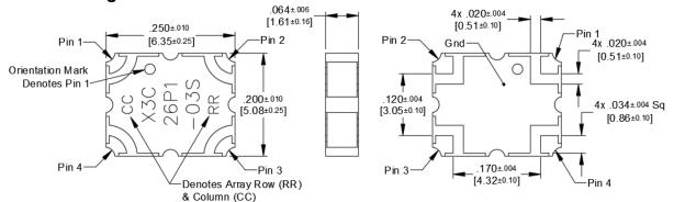
Dimensions are in Inches [Millimeters] X3C26P1-03S Mechanical Outline Tolerances are Non-Cumulative
