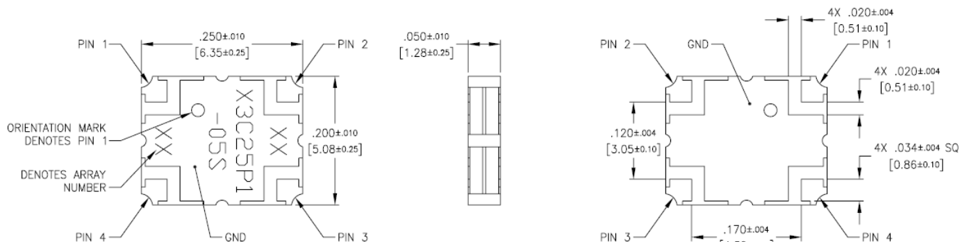
Dimensions are in Inches [Millimeters] X3C25P1-05S Mechanical Outline
