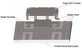
Figure 4: Mounting Features Example
