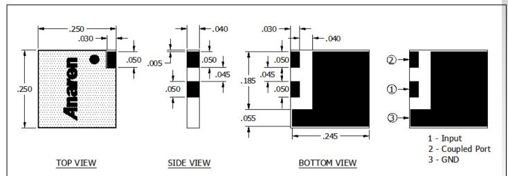
Tolerance is  $\pm 0.010$ ", unless otherwise specified. Designed to meet or exceed application portions of MIL-E-5400. **All dimensions in inches.**
