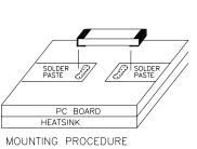
Make sure that the devices are mountd on flat surfaces (0.001" under the device) to optimize the heat transfer.
