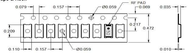
DESPOOLING DIRECTION — FARE DETAIL & RF PAD ORIENTATION
