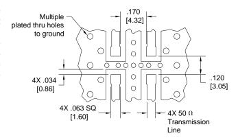
Dimensions are in Inches [Millimeters] 1P510\* Mounting Footprint
