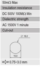
Rating 3A 125V AC 1.5A 250V AC Contact resistance
