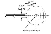
Piezoelectric Buzzer External Drive)
