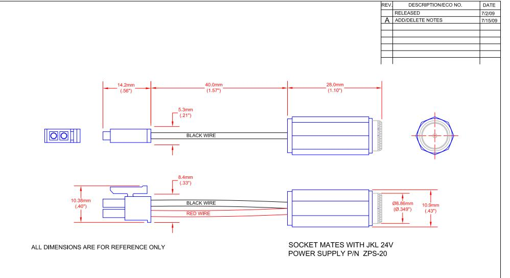
INPUT CONNECTOR MATES WITH JKL ZAF ALUMILINE SERIES LED LIGHT BARS.
