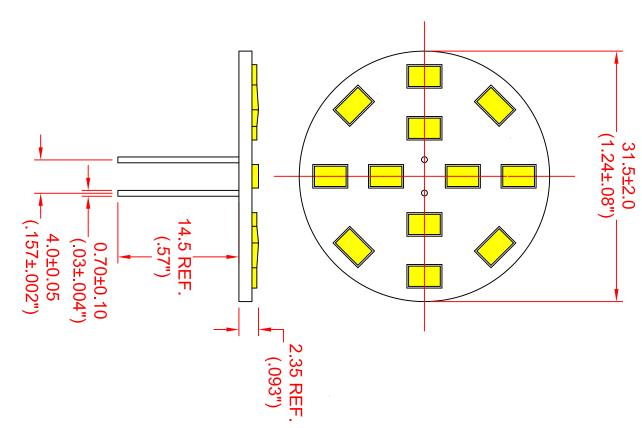
NOTE: OVERALL THICKNESS OF ASSEMBLY IS LESS THAN 11mm (.433").
