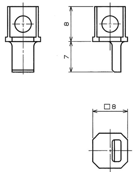
NOTE 1. BOTH QE-POL-POST AND QE-POL-KEY ARE PROVIDED WITH SCREW, NUT AND SPRING WASHER.
