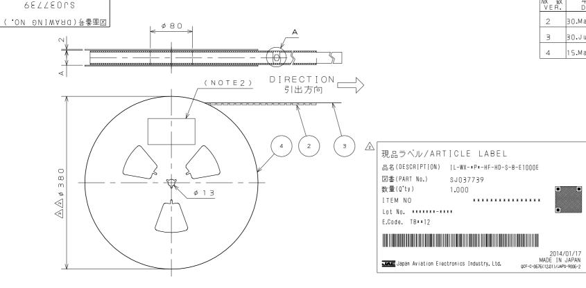
NOTE1. SUFFIX "-E1000E" OF THE PART NUMBER INDICATES THAT 1000 PCS. OF IL-WX-\*P\*-HF-HD-S-\*E" CONNECTORS ARE ACCOMMODATED IN 1 REEL.
