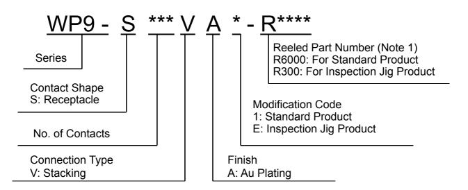
Note 1) An embossed tape reel contains 6,000 pieces of standard product, or 300 pieces of inspection jig product. Please contact us for details on embossed tape specifications.
