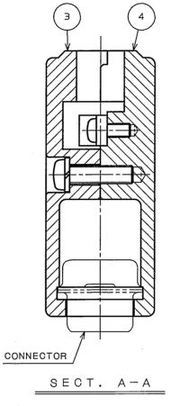
NOTE 1.APPLICABLE CABLE DIAMETER SHALL BE  $\phi$ 5.5 $\sim$  $\phi$ 7. CABLE DIAMETER SHOWN HERE IS WHEN THE SHIELD IS BENT.
