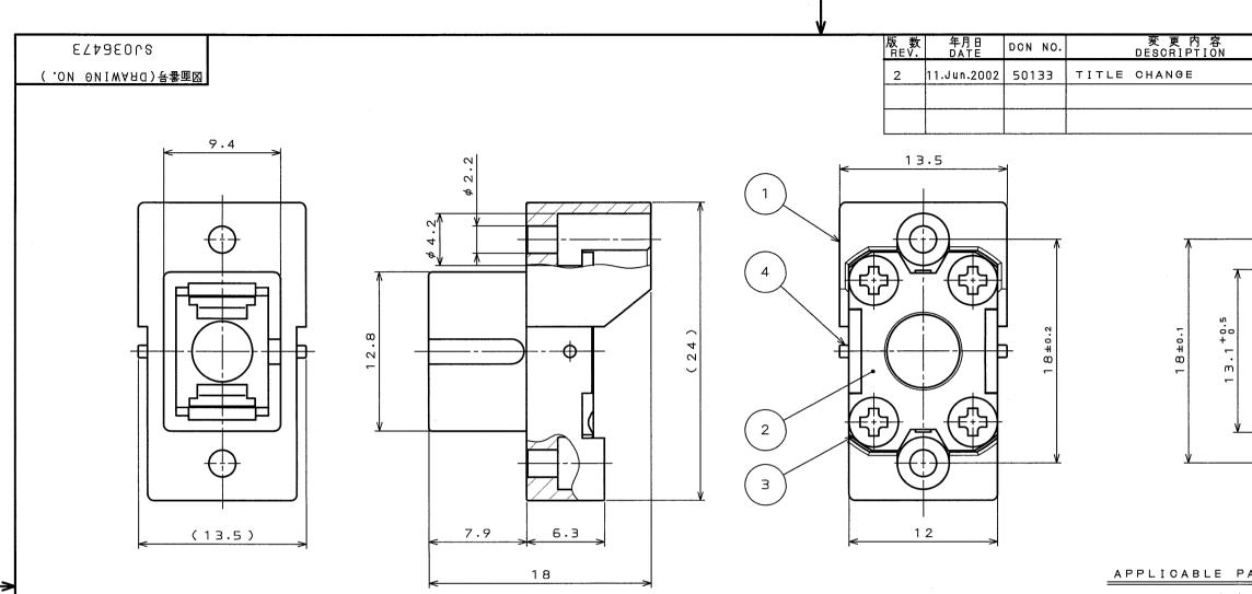
▲NOTE1.Do not apply the load larger than 19.6N to when SC connector is mated with FO-SC-RS-N
