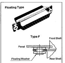
The floating washer moves .030 in. (0.4 mm) in any direction relative to the center (  $\P$  ).
