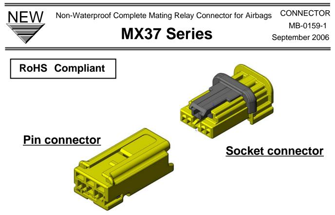
This non-waterproof compact relay (inline) connector was developed for automotive air bags. It has a structure which separates the connection of the contacts with the repulsion of the coil spring when the connectors are not mated completely (mechanical perfect mating design). Furthermore, the built-in short contact (short circuit) prevents malfunction due to static electricity when the connector is not mated.
