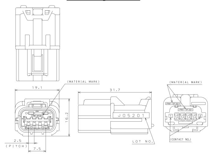
For 2pos. (MX36002PQ3) only the rear cover(shape, color) will be different (SJ Drawing SJ101630)
