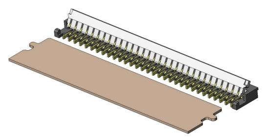
The FB10-JT1 Series is a 0.3mm pitch, low profile, bottom-surface connection type FPC connector ideally suited for ever-smaller portable devices such as smartphones, tablet PCs, and digital cameras.
