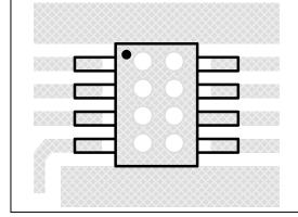
Figure 36 Board Via Layout For Thermal Dissipation
