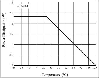
Figure 35 Dissipation Curve
