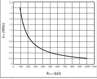
Figure 30 Operating Frequency vs. R<sub>TON</sub> Resistance
