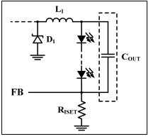
Figure 29 Adding Output Capacitor
