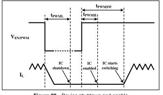
Figure 28 Device shutdown and enable
