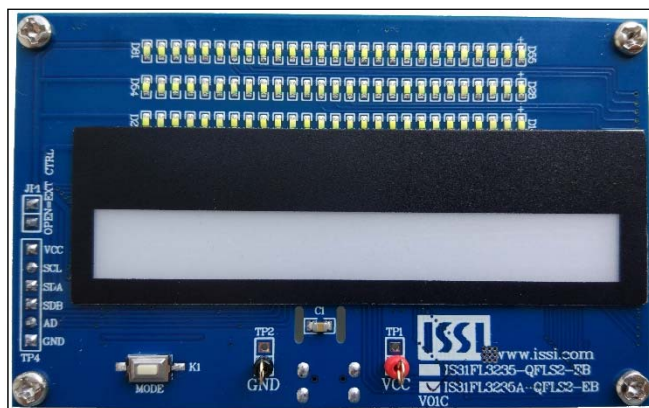
Figure 8: Photo of IS31FL3235A Evaluation Board (LPC922 Version)
