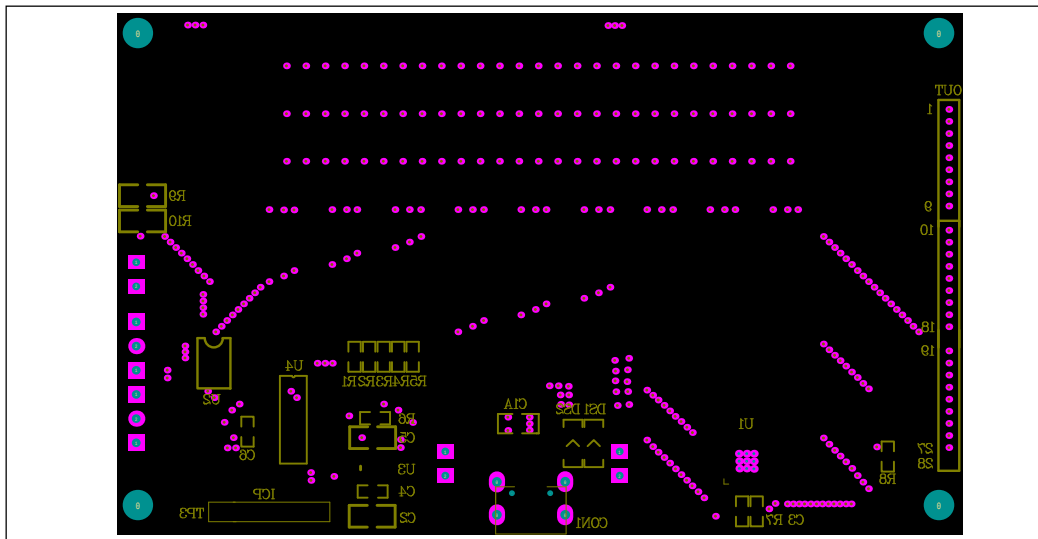
Figure 13: Board Component Placement Guide - Bottom Layer
