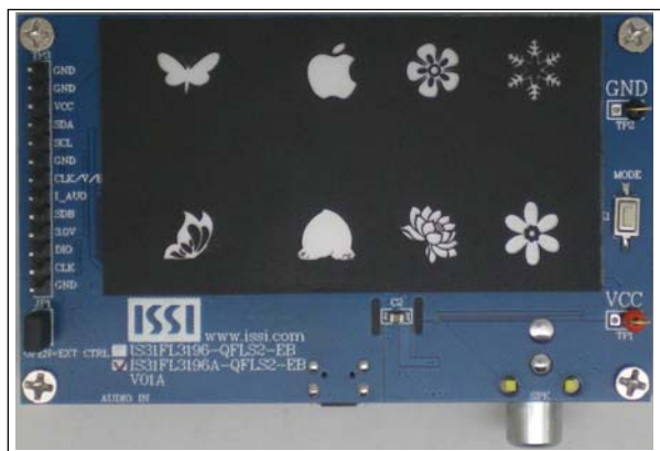
Figure 1: Photo of IS31FL3196A Evaluation Board
