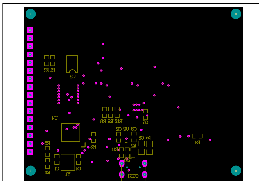
Figure 5: Board Component Placement Guide - Bottom Layer
