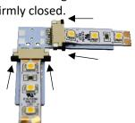
4 Insert strip into the gap between black sliding latch and beige bridge piece, matching polarity of strip to (+) signs on Tiger Paw® board.
