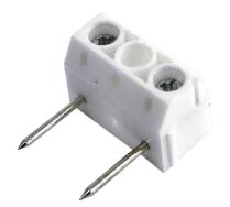
Inspired LED's **Solderless 2-Prong Screw Terminal** pairs with our Infinity Series Weather Resistant LED Dura-flex, terminating bare ends to cable. Sturdy prongs pierce the copper wiring on either side of flex to create a secure connection, while screw terminals allow cable to be run from strip to strip, or directly to power source.
