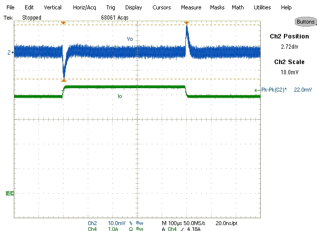
Transient response-Sourcing mode Vin-1.35V Vout-0.675V/3.9-4.3-3.9A Ch4-Vout Ch3-Iout (1A/μSec slew rate)
