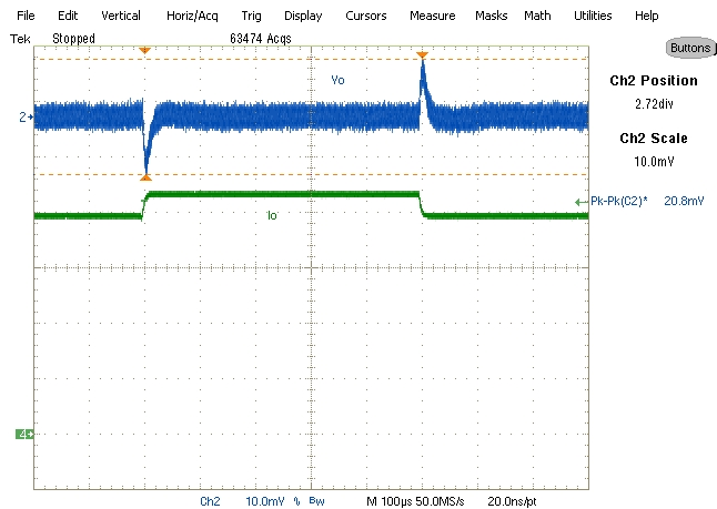
Transient response-Sourcing mode Vin-1.5V Vout-0.75V/3.9-4.3-3.9A Ch4-Vout Ch3-Iout (1A/μSec slew rate)
