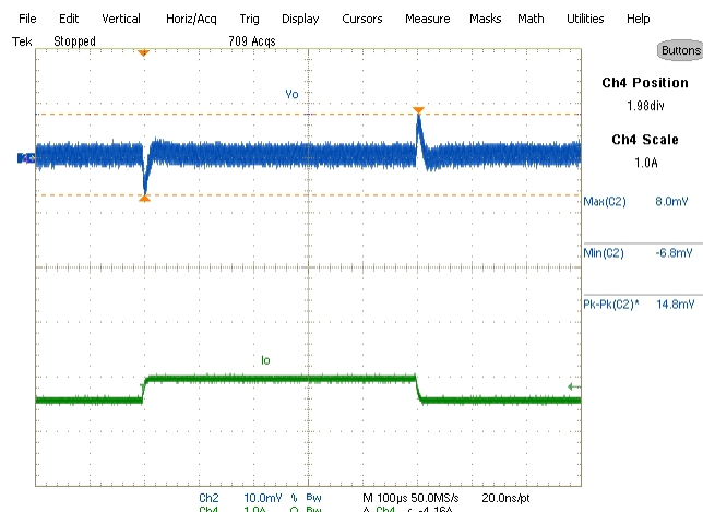
Transient response-Sinking mode Vin-1.5V Vout-0.75V/3.9-4.3-3.9A Ch4-Vout Ch3-Iout (1A/μSec slew rate)
