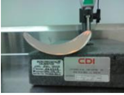
Fig.2 Wafer pre-solder of 70 \mu\text{m} IGBTs showed a severe warpage of 32 mm.
