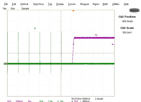
Figure 34: Short circuit (Hiccup) Recovery, Ch3: V_{out} , Ch4: I_{out}
