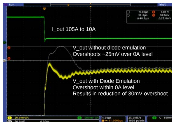
Figure 7: Output voltage overshoot reduction with body-braking
