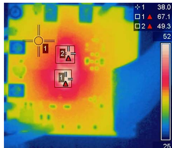
Figure 22: Thermal Image at V_{IN} = 19V , I_{OUT} = 6A (IR3473: 67^\circ C , Inductor: 49^\circ C , PCB: 38^\circ C )
