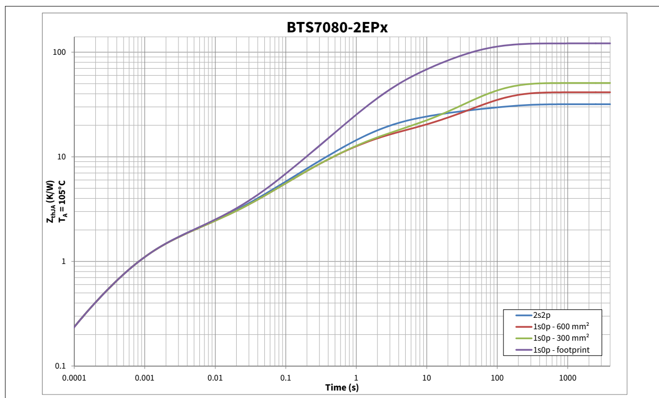
Figure 9 Typical Thermal Impedance. PCB setup according Chapter 4.4.1
