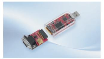
The UConnect XC2000 is a low-cost Starter Kit that provides full evaluation capability for the new XC2000 16-bit family of microcontrollers. The kit includes development toolchains, demos, a EB TRESOS studio for driver configuration and tutorials for quick installation and ease-of-use. The Uconnect USB stick comes with a CAN extension board.
