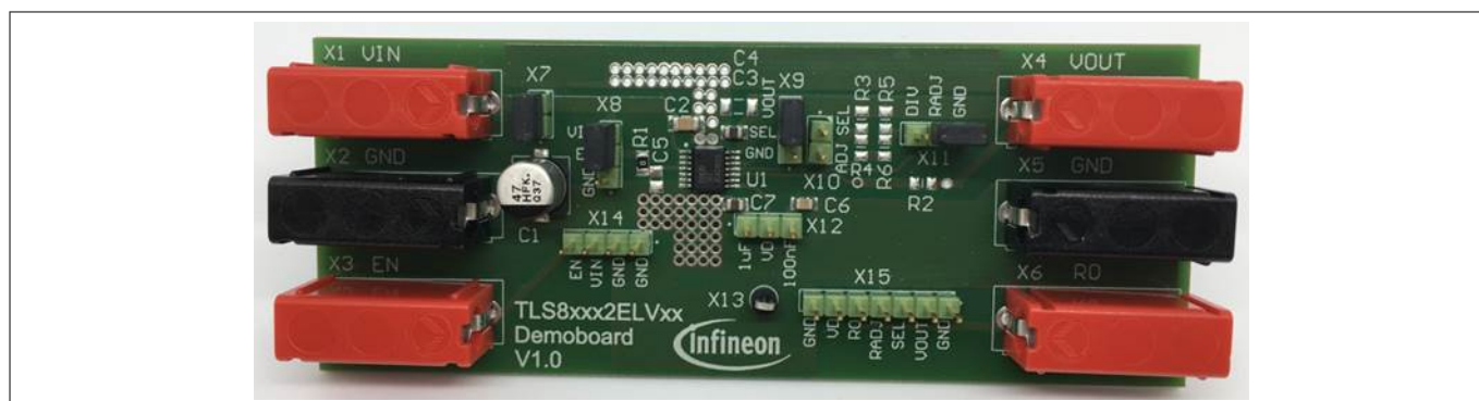
Figure 4 TLS835B2ELV default jumper setting
