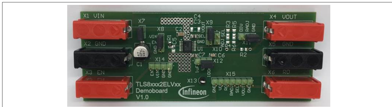
Figure 3 TLS820D2ELVSE, TLS835D2ELVSE default jumper setting
