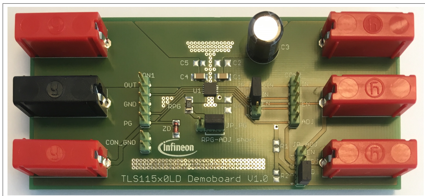
Figure 3 OPTIREG™ linear voltage regulator TLS115x0LD demoboard
