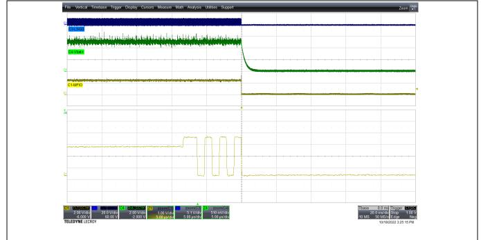
Figure 25 Vout\_UVP triggering at overload of 3.3 Ω resistor at the output
