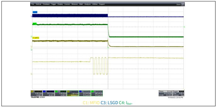
Figure 23 OCP1lev2 triggering at output load of 4.7 A
