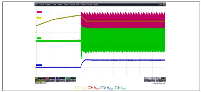
Figure 17 Start-up at full load, 230 V AC input
