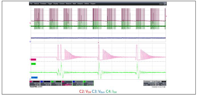
Figure 21 Burst mode at VBat+ = 40 V, load = 0 A, CCset: 0 V
