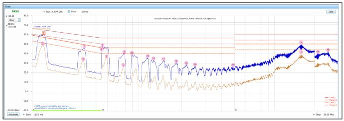
Figure 15 Conducted emissions – phase line
