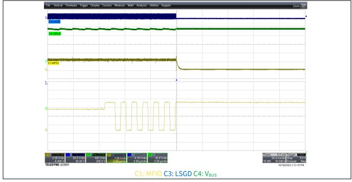
Figure 24 Vin\_OVP triggering at input voltage of 268 V AC
