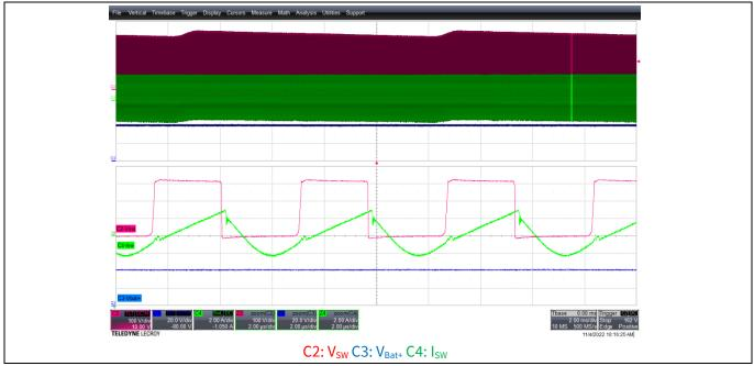
Figure 19 CRM mode at VBat+ = 40 V, load = 4 A, CCset: 3.07 V
