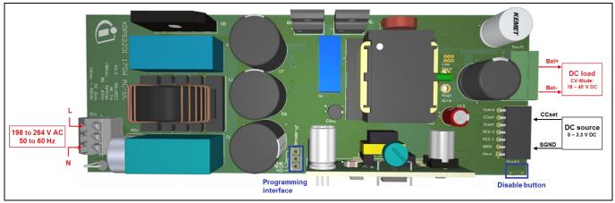
Figure 2 CC test setup with electronic load and setting CCset via DC source
