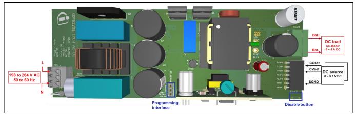
Figure 3 CV test setup with electronic load and setting CCset via DC source
