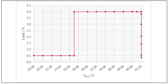
Figure 11 CC-CV charging behavior, Iload = 0.5 A and 4 A, CCset = 0.42 V and 3.05 V, CVset = 3.0 V
