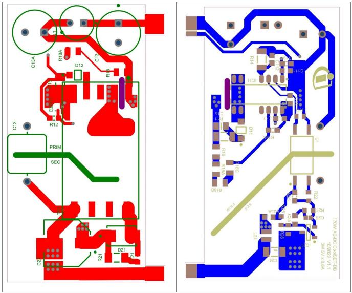
Figure 9 CoolSET<sup>™</sup> daughterboard PCB top (left) and bottom (right)
