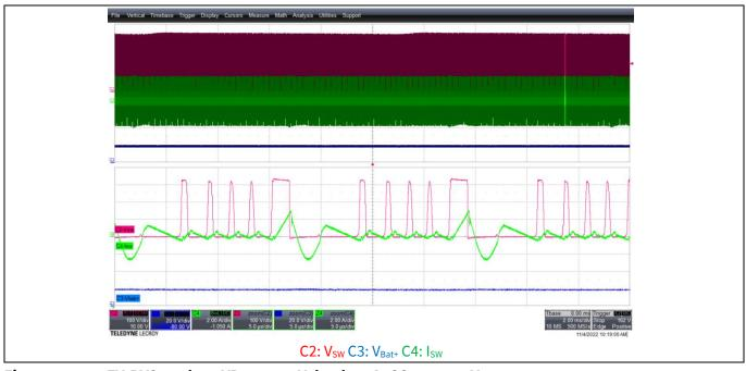
Figure 20 ZV-RVS mode at VBat+ = 18 V, load = 2 A, CCset: 1.54 V
