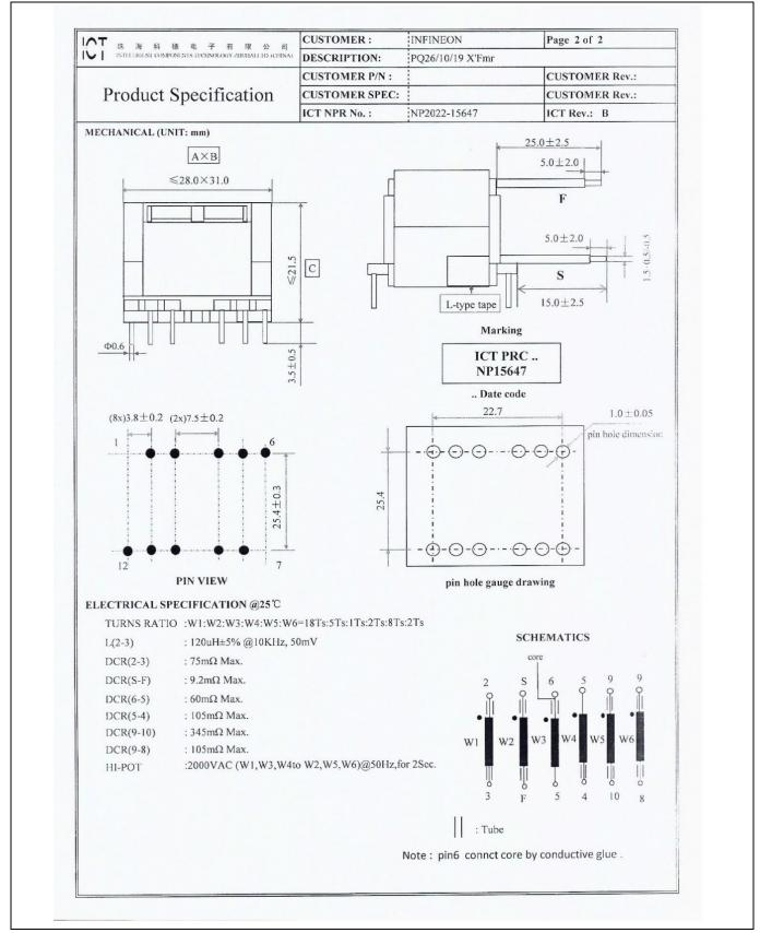
Figure 26 Transformer specifications of NP2022-15647-B
