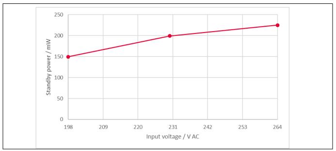
Figure 12 Standby power consumption
