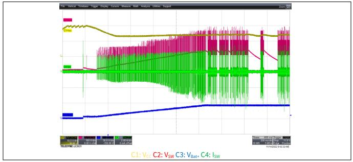
Figure 18 Start-up at no load, 230 V AC input
