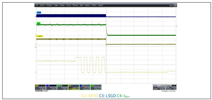
Figure 22 OCP1lev1 triggering at output load of 4.4 A
