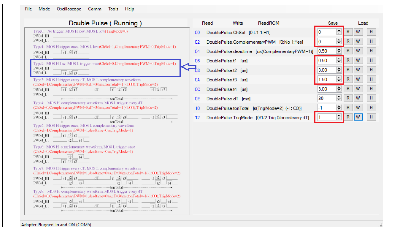
Figure 18 Trigger once mode configuration for the low side MOSFET
