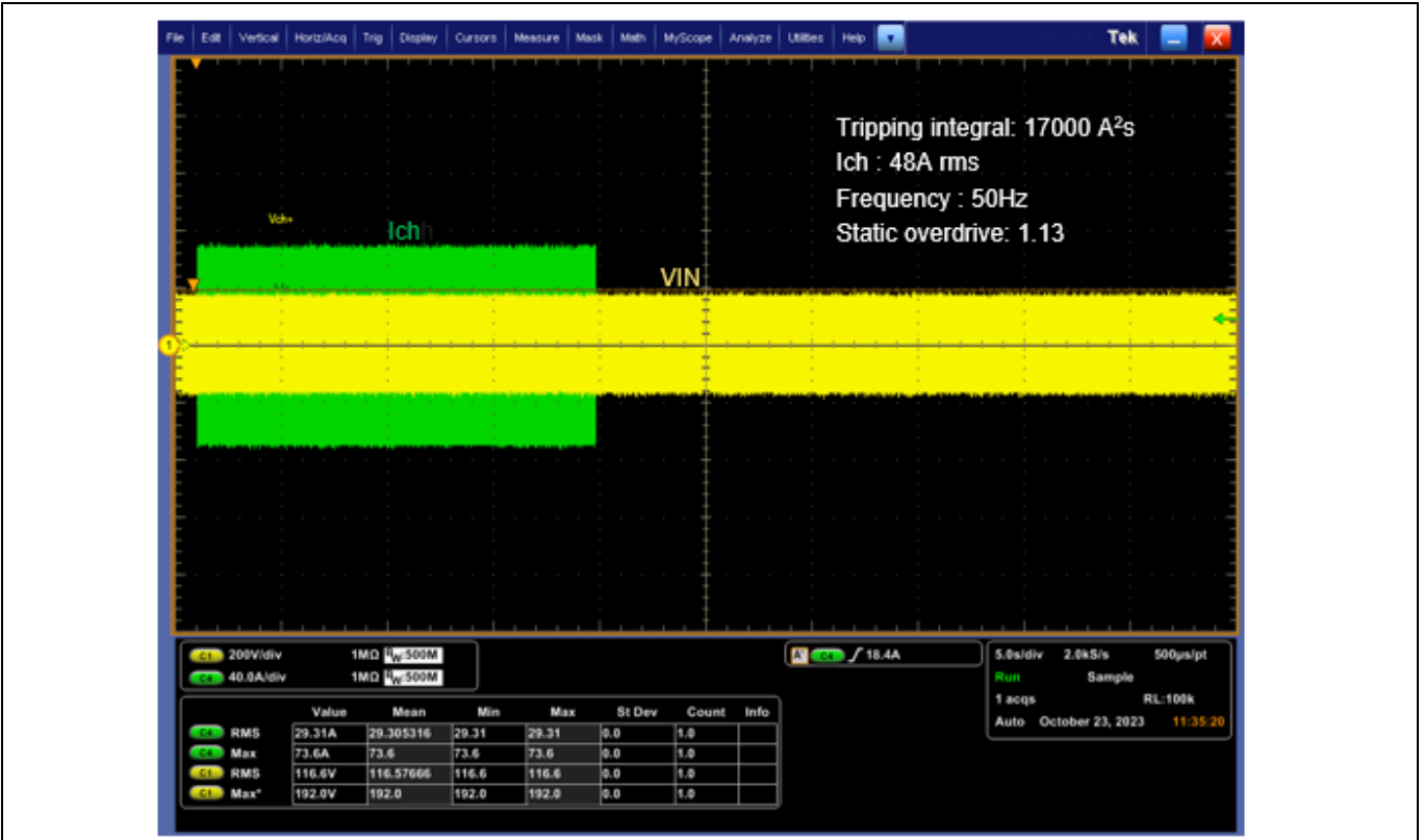
Figure 20 OVL integ test
