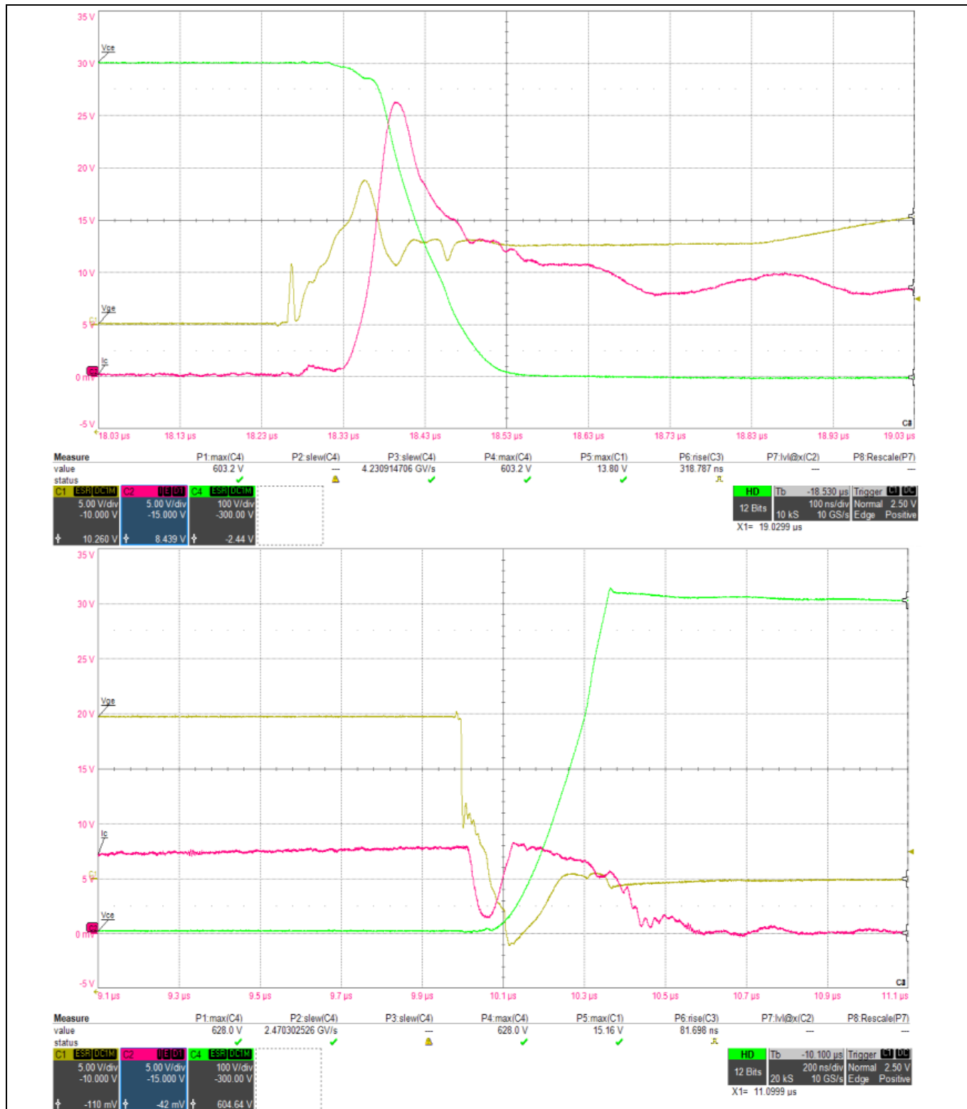
Figure 6 Turn-on (top) and turn-off (bottom) of IKQ75N120CT2 as low-side switch ( V_{DC} = 600\text{ V} , I_C = 7.5\text{ A} , /INF = 1 ; yellow: V_{GE} 5 V/div, red: I_C 5 A/div, green: V_{CE,LS} 100 V/div)
