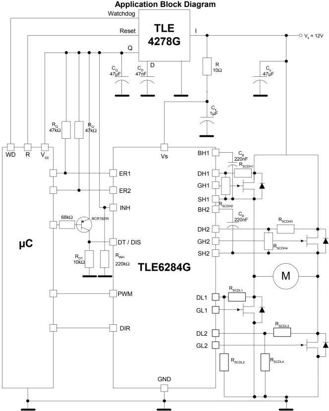
This application block diagram shows one of the possibilities to use this Driver IC. The voltage divider networks accross the 4 MOSFETs (resistors  $R_{SCDxx}$ ) allow to increase the current limit threshold for Short Circuit protection. The  $R_{SCDLx}$  resistors also provide a charge path for the bootstrap capacitors. If  $R_{SCDLx}$  resistors are not used in the application, a 12k Ohm resistor should be introduced between SH1 to GND and SH2 to GND.
