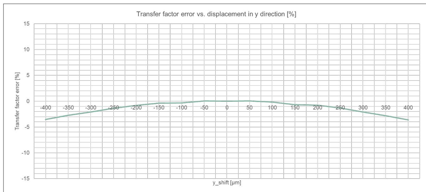
Figure 20 Transfer factor error due to sensor displacement in y direction
