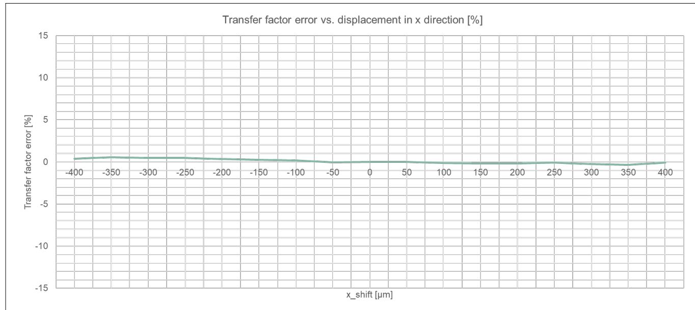
Figure 19 Transfer factor error due to sensor displacement in x direction
