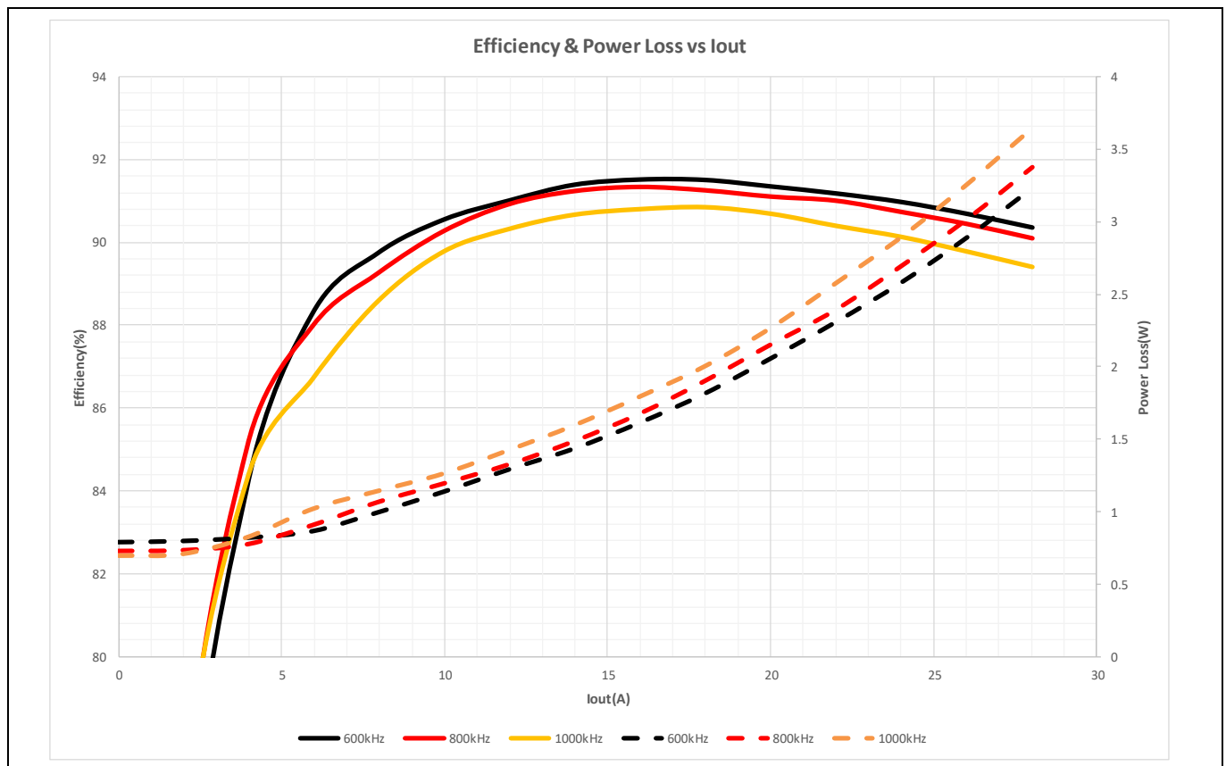
Figure 6 Typical efficiency and power loss curves, PV_{in} = 12\text{ V} , F_{sw} = \text{Varying}
