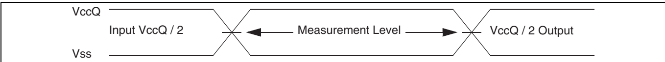
Figure 25 Input waveforms and measurement levels [64]
