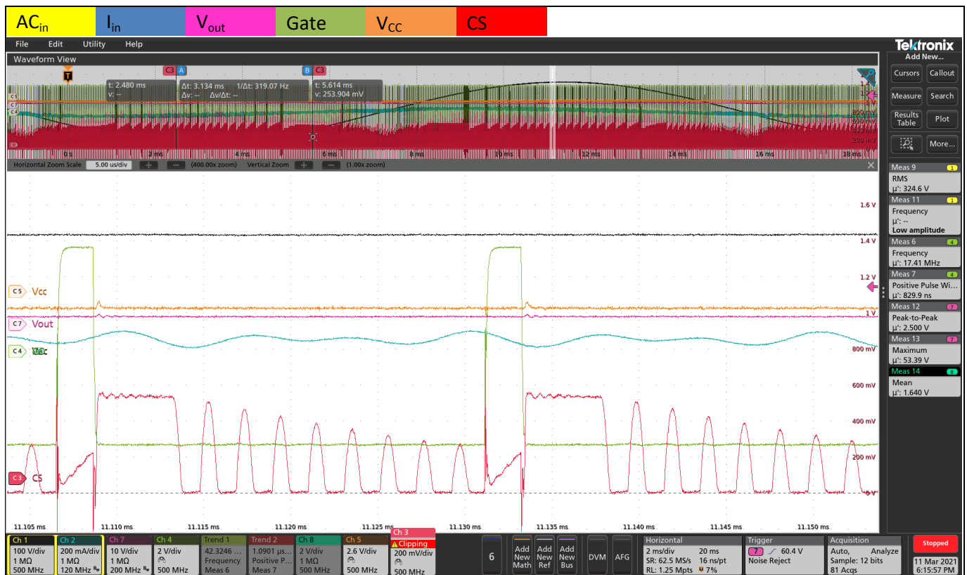
Figure 32 230 V ninth valley operation ( V_{out} ripple pk-pk 2.5 V)
