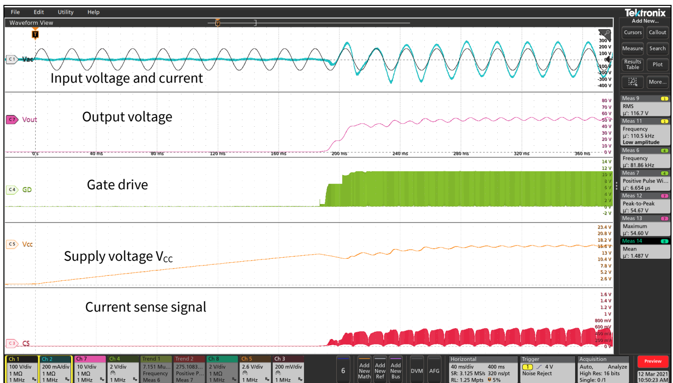
Figure 27 Start-up at 120 V at full load
